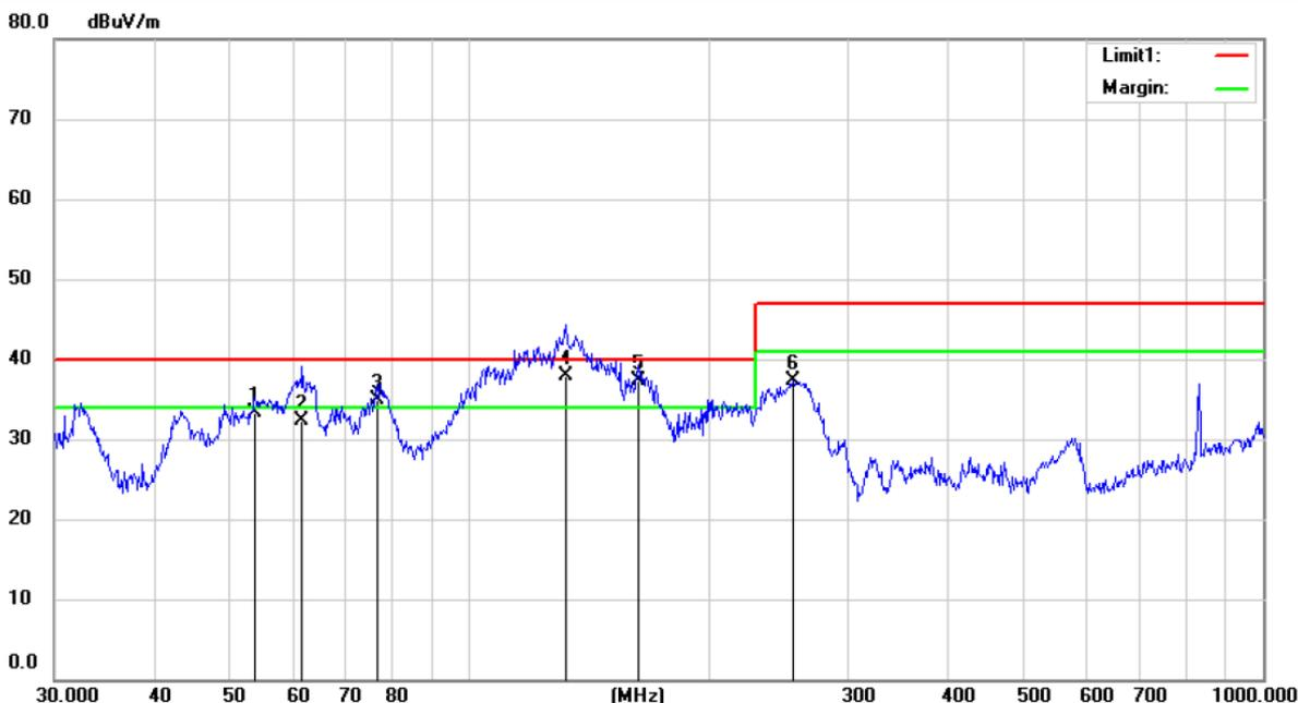
Site: 3m Chamber #3      Polarization: **Vertical**      Temperature: 22.5 C
